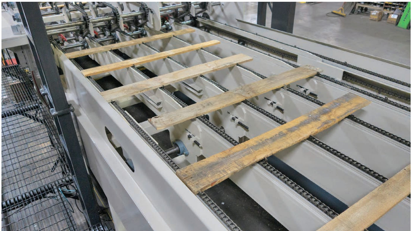
Optimized Trim Saw System: The scanned boards are logged, optimized to the chosen cut/sort recipes selected and then presented to the saw module. This approach helps optimize yield better than a human operator can and ensures consistency and accuracy of cuts.
