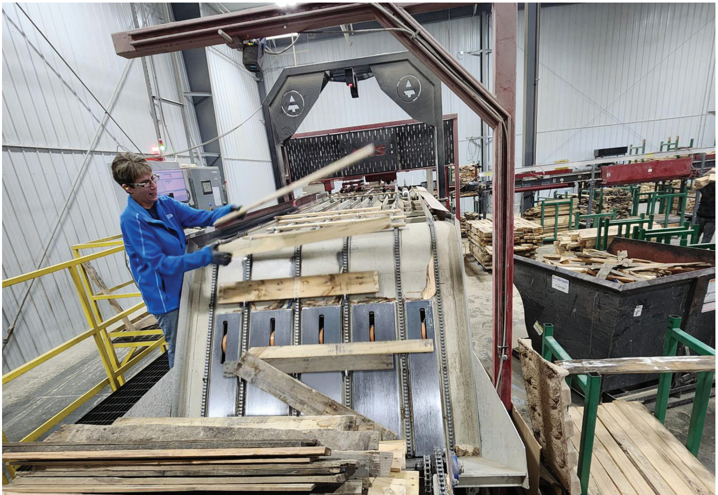
Berry Pallets selected the Auto-Max because of the footprint size of the unit, the production capability and the relative safety of the line compared to manual trim saws. Berry Pallets uses the Auto-Max to process both new and recycled boards.
